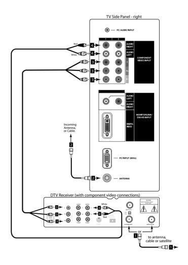
Figure 11. Connecting the DTV receiver with component Video Connections.
